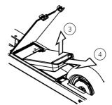
Rotate the 2 locking knobs to unlock, then pull up the cover to reveal the battery.
