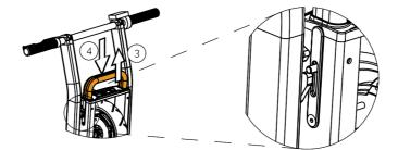
As you pull the rear frame closer to the handlebar, pull the handle up. Notice the 2 pins sticking out from the side of the frame, let the pins sit into the slots on the steering column.
