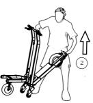
Give a kick to the upper pedal as indicated to unlock the locking mechanism. (Worry not of kicking too hard, MIMO C1 is built to withstand moderate abuse!)
