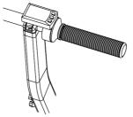
There are 2 buttons on the thumb throttle. Press and hold top button to switch MIMO C1 on, and use bottom button to select speed modes.
