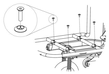
Use the supplied screw and washer to change different rack module.
