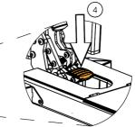
Without standing on the board, gently step on the lower pedal to secure the locking mechanism.
