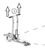
Pull the handlebar upwards so the initial locking will sit into place.
