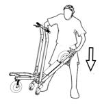
One hand in the middle of the handlebar, one hand lower the rear frame till the rear wheel touch ground.
