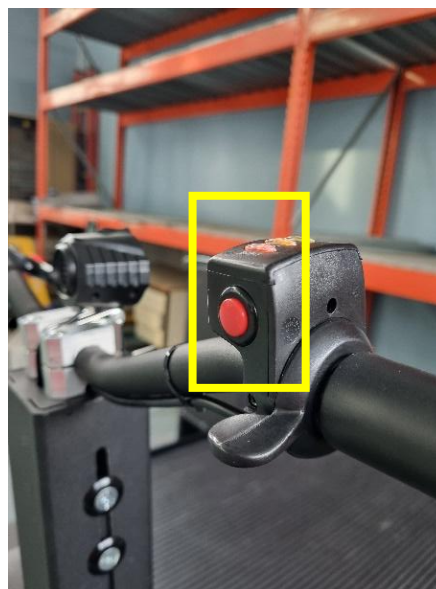
Fig.6: Button pressed = reverse mode!
