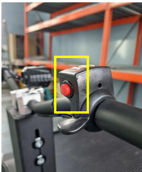
Fig. 5: Button out = forward mode!
